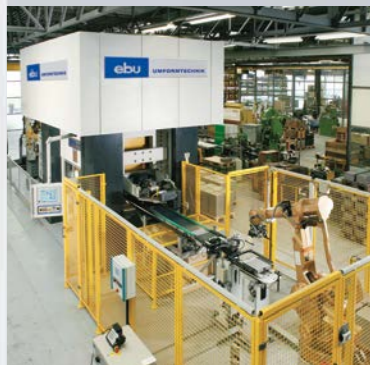
In line of duty in a furniture maker's facilities – automatic ebu punching press with robot and depiling system
